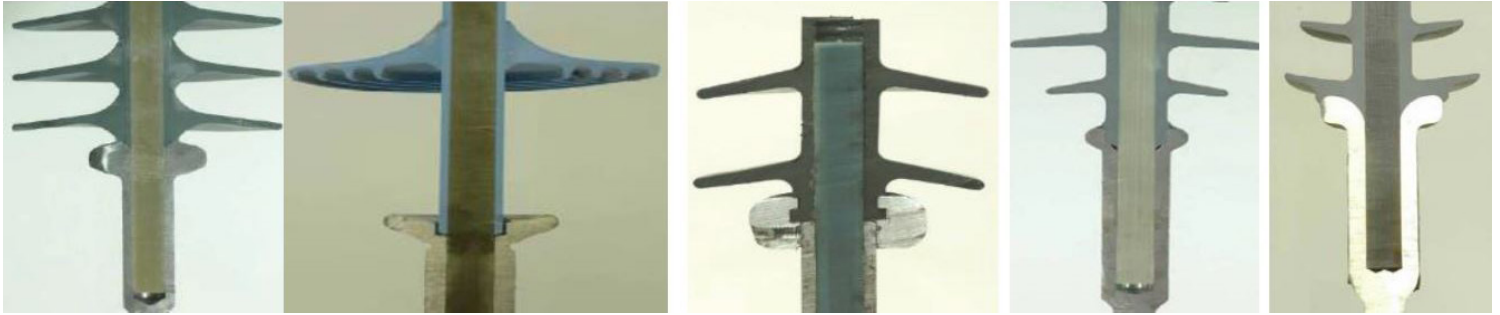
Figure 1: Typical designs of composite insulators
