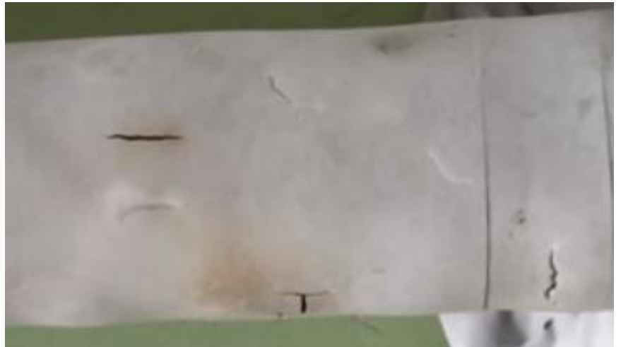
Figure 21: Cracks in silicone housing left after being subjected to heat for a few hours
