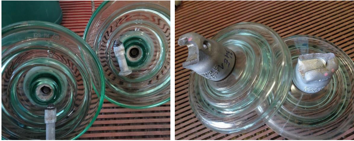
Figure 17: Typical aspect of the glass units after the test
