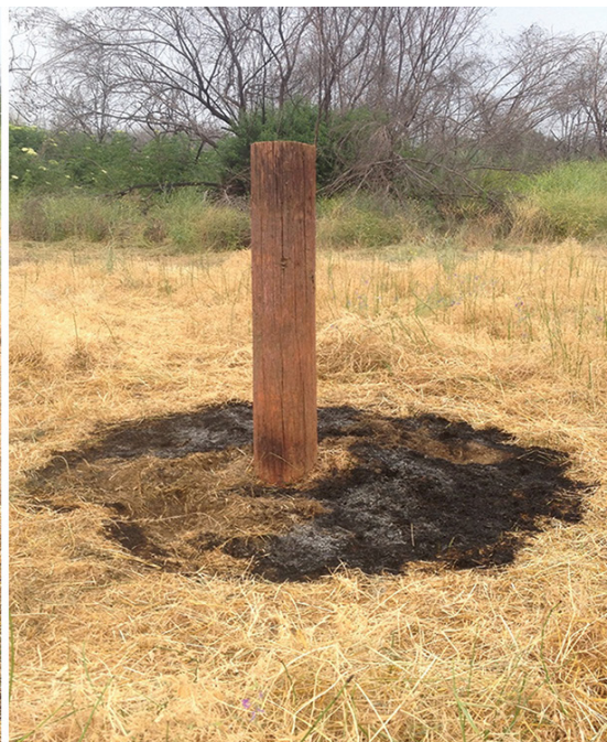
Results of a controlled live fire where dry vegetation stacked around the pole burned and ignited an untreated pole. The pole had to be extinguished (left). Results of a controlled live fire where dry vegetation stacked around the pole burned but did not ignite or damage the pole pretreated with long-term retardants (right).
