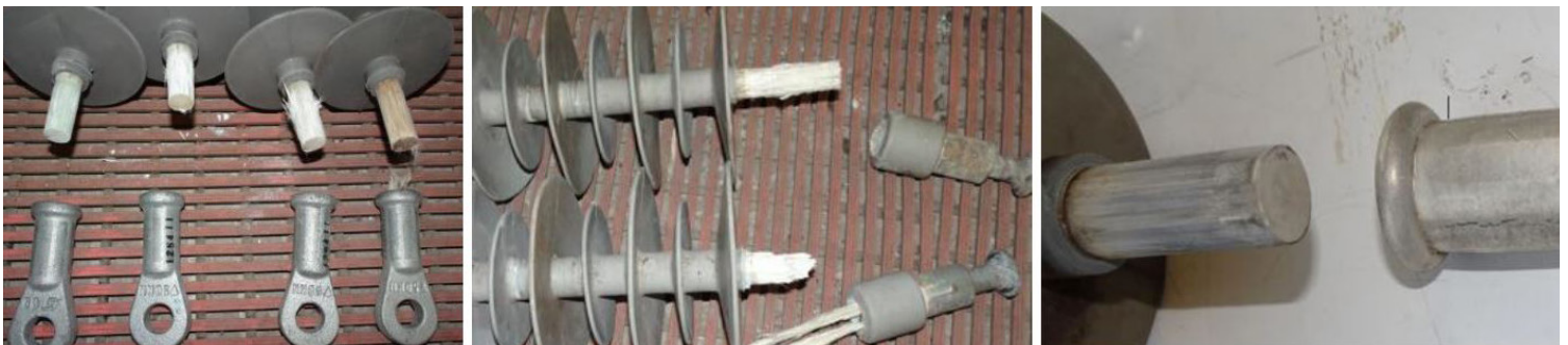
Figure 12: Typical aspect of the tested units after the mechanical pull test
