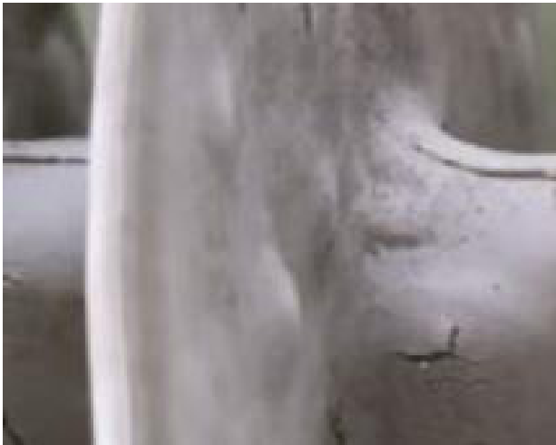
Figure 21: Cracks in silicone housing left after being subjected to heat for a few hours
