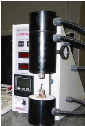
Figure 2: Torsional strength test showing the loss of resilience at the Tg set point
