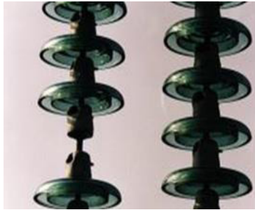
Figure 9: Typical aspect of a "stub"
