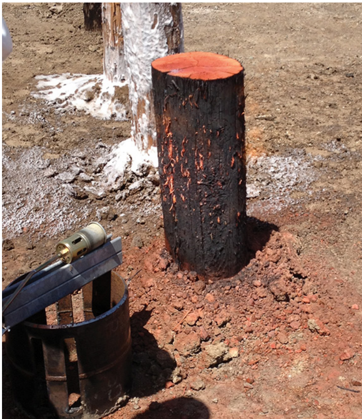
Pole pretreated with long-term retardants exposed to a flame from a propane burner at more than 2000°F (1093°C) did not ignite or show any damage.
