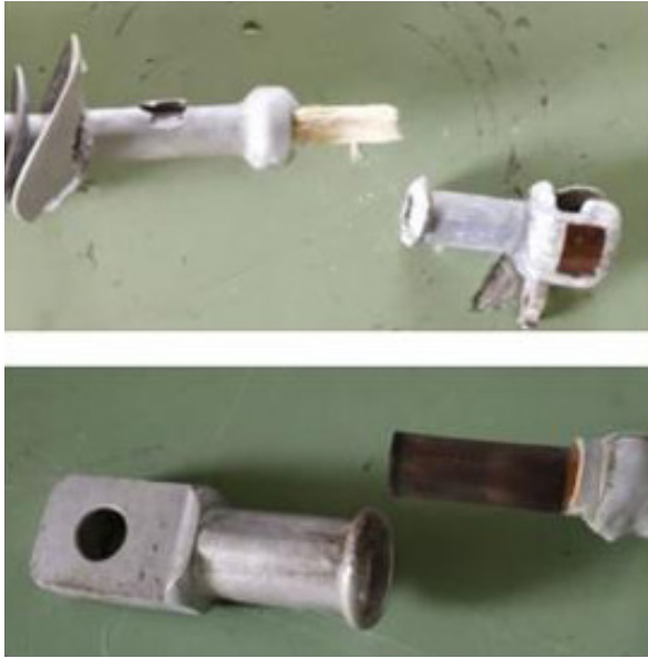
Figure 20: Fitting pull out after the insulators were cooled down after a heat cycle at 300°C and comparison with results on glass stubs tested in the same conditions
