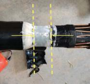
Case Study 2 common splice installation defect type 2: Uncentered splice body. No gap (left) and too large of a gap (right) which misalign the stress control and yield voids under the splice body and result in substandard
