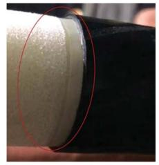
Damage to the insulation (off white groove) introduced during the outer semiconducting layer (black) cutback at a separable connector (T-body) termination with substandard performance (per IEEE 386) from Case Study 1.
