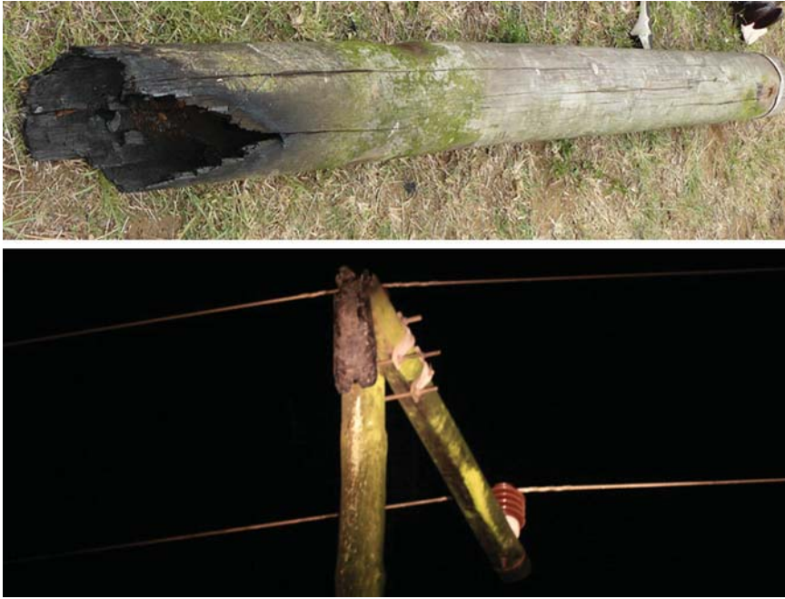
Examples of unbonded cross arms that burned (top). Example of tracking on unbonded cross arm (bottom). Photos by Eskom.
