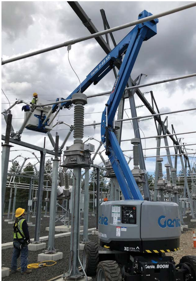
Articulated boom lifts, like Genie's Z-45 XC, provide 24 feet of up-and-over capability, a maximum 1,000-lb platform capacity, a 5-foot jib for precise positioning, and zero tail swing. Photo by Avista Utilities.
