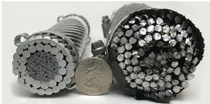
New ACCR conductor compared to original ACSR conductor. Courtesy of 3M.
