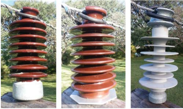
Design-acceptable insulators for mounting phase conductors: capped porcelain, uncapped porcelain with collector plate and capped composite insulator. Photos by Eskom.
