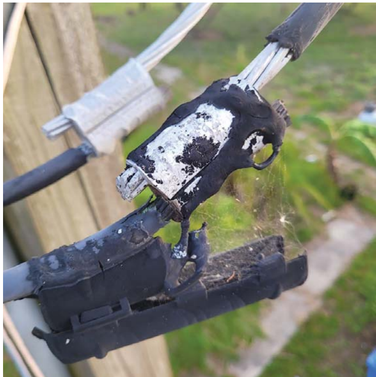
An example of high impedance; a bad hot leg connector. Photo by ComEd and Itron.
