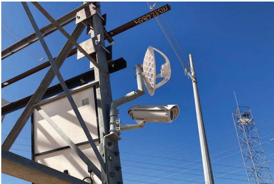
Through artificial intelligence, the cameras learn the surrounding environment, report changes and provide alerts when identifying smoke from wildfires or changes to structures. Photo by Salt River Project.
