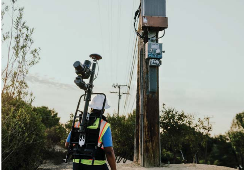
Osmose crew member using backpack OsmoVision technology to capture pole data that will be used in the pole loading analysis. Photo by Osmose.
