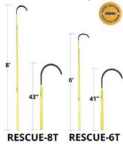
Designed to comply with OSHA 1910.269(j) for the construction of live line tools and OSHA 1926.957 for the use of live line tools. the Saf-T-Gard Voltgard **Telescopic Insulated** Rescue Body Hooks are coated and heat treated with an 18" hook opening and mounted on a 6' or 8' telescopic fiberglass handle to safely withdraw injured personnel from confined spaces, in vaults, near electrical cabinets or switch gear. The unique retractable design potentially saves
