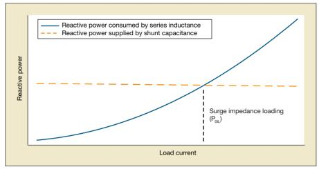
Transmission line reactive power balance as a function of load current.
