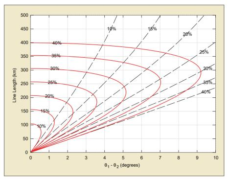
Contour plots of (1) and (2) superimposed for the underground transmission line of the power system shown in the bottom figure on page 43 as a function of both line length and voltage phase difference. The numbers on the graph represent the total apparent power (solid red lines that curve back on themselves) and real power (dashed black lines which extend upward) expressed as percentages of the surge impedance limit.
