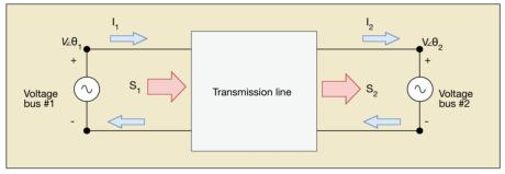
Simple power system used to determine length limits for underground cable.
