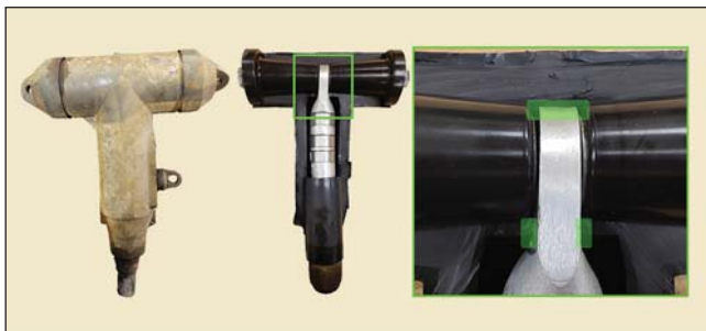
Surface contact problem with T-elbow. Graphic by Hydro-Quebec.
