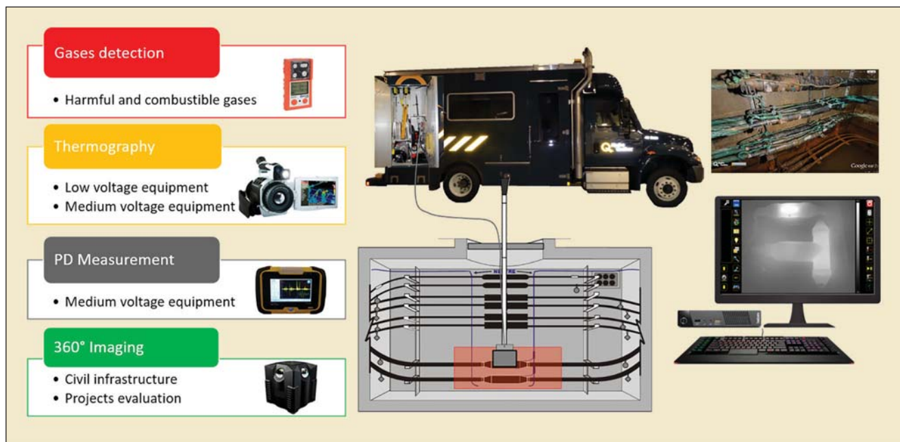
Inspection program phases. Graphic by Hydro-Quebec.
