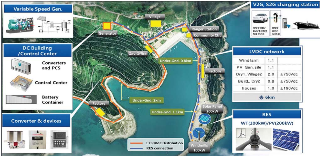
ARABIC 1, in the section titled “DC Distribution System”. Configuration of low-voltage dc distribution system on an island.
