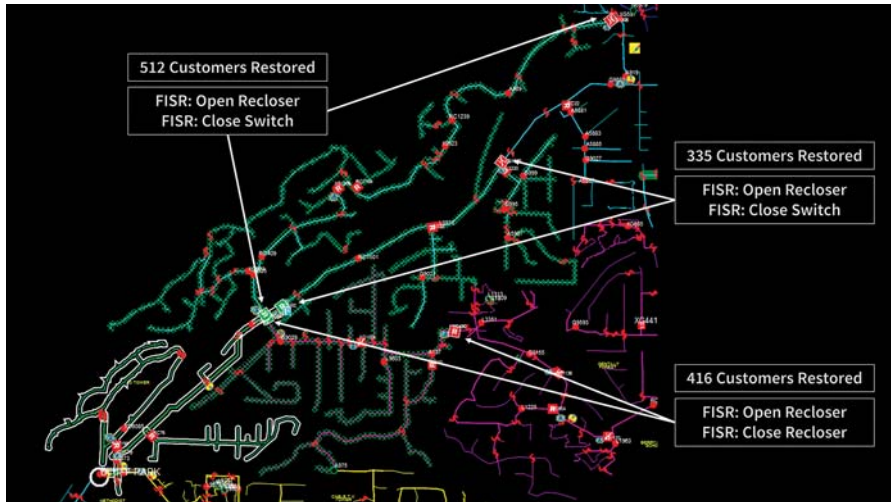
Feeder breaker outage on Bluff Park substation. FISR implemented a 6-step plan to restore 1,263 of 1,630 customers within 110 seconds of FISR starting evaluating, 48 seconds of which was just sending SCADA controls.
