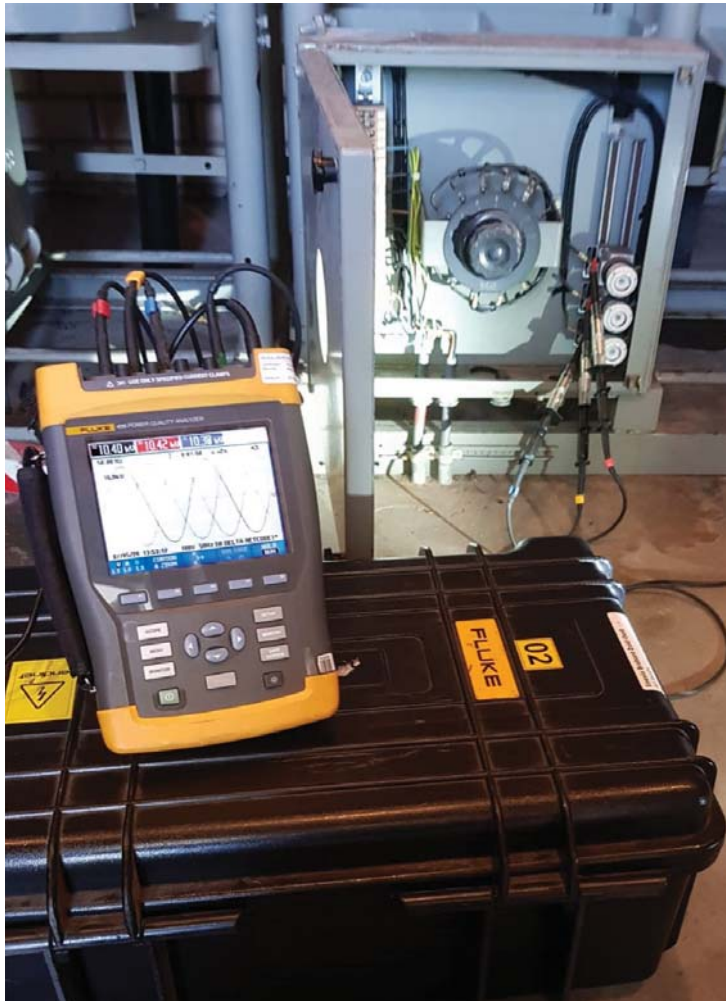
Field measurements for national level PQM campaign using Fluke 435-II meter.
