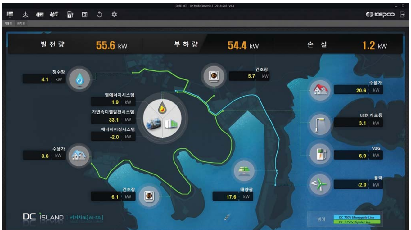
ARABIC 2, any placement in final two sections. Human-machine interface screen of low-voltage dc operation system.
