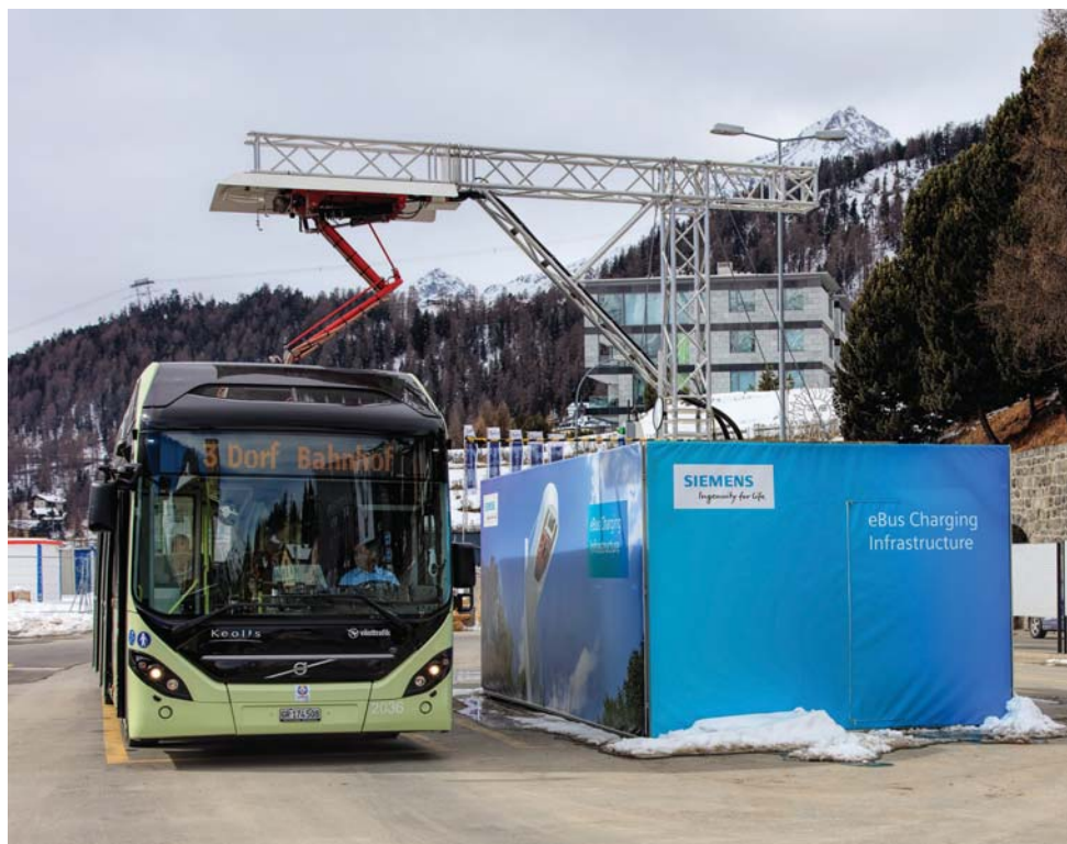
A Volvo 7900 Electric Hybrid bus at the quick-charge facility on Bahnhofplatz Square in Zurich. Buses of this type use electrical power coming from accumulators for normal operation mode and can switch to a traditional engine if necessary. Credit: Denis Linine, Dreamstime
