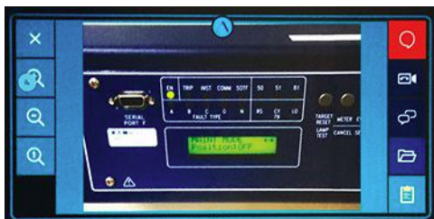
The Atheer Air O&M app consists of instructions, pictures and videos associated with settings change on an SEL 351A substation relay to put it into maintenance mode and then return it back to normal mode.
